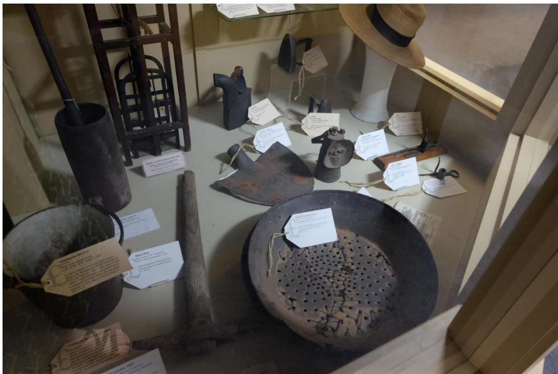
Figure 21: Mining items featured in display, right to left, top to bottom. Iron Dolly Pot, Model of miner's safety cage, amalgam bucket, short pick, paddler shovel (centre), two miner's candles with spikes to insert into rock, gold panning dish. Various ages and donors.
