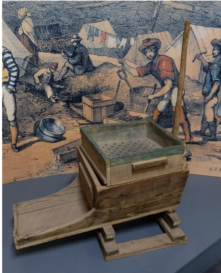
Figure 20: Gold cradle - sat on wooden frame on 2 rockers, cloth on shelf coir matting and extended metal on floor for gold saving, an adaption of ancient sluice box by the addition of rockers and shelves (M1067), donated prior to 1975.
